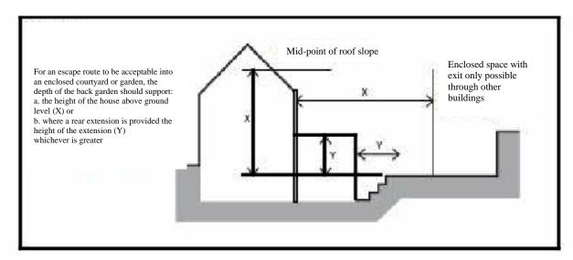
Where it is not practical to provide such access, for instance where the exit from the basement passes through a kitchen or shared living room a secondary means of escape must be provided.
